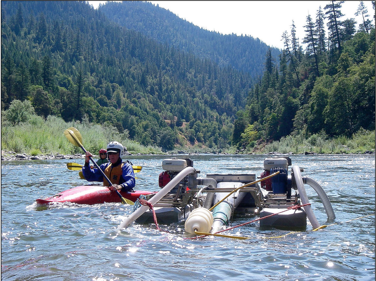
Photo 2: Whitewater kayakers paddling in immediate proximity to a dual-engine, dual-nozzle suction dredge discharging effluent into the Klamath River, July 2008. The dredge is placed such that kayakers must paddle through its effluent to reach the top of the eddy and access the river's current. Both dredge operators are operating the nozzles underwater.
