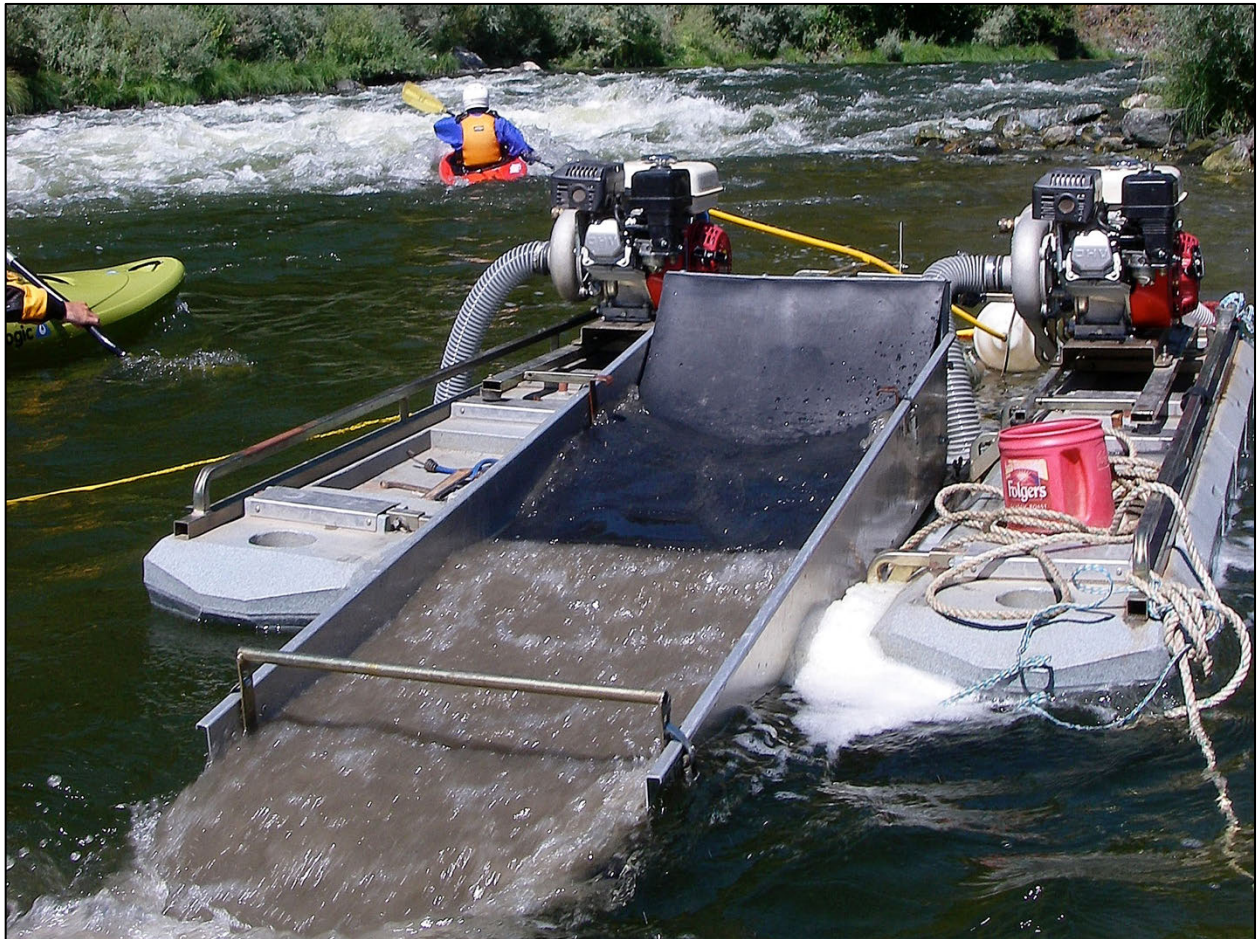
Photo 1: Whitewater kayakers paddling in immediate proximity to a dual-engine, dual nozzle suction dredge discharging effluent into the Klamath River, July 2008. The dredge is placed such that kayakers must paddle through its effluent to reach the top of the eddy and access the river's current. Both dredge operators are operating the nozzles underwater.
